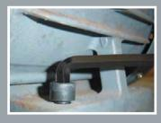
Tighter inside radius means full smooth entry into screw head.
